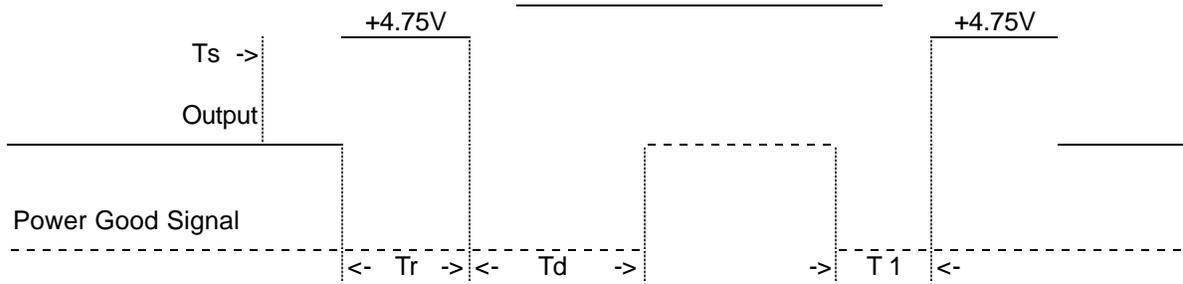
Note:  $T_r \leq 100$  ms,  $T_1 \geq 1$  ms,  $T_d = 100 - 500$  ms.
